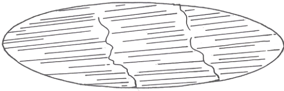
Sketch of PSF on bedding plane with parallel slicken striae disrupted by microscale "steps" or "asperities"
